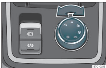
Fig. 205 Consola central: Mando rotativo (Driving Experience button).
