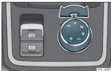
Fig. 205 Consola central: Comandament rotatiu (Driving Experience button).
