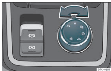
Fig. 205 Consola central: Comandament rotatiu (Driving Experience button).
